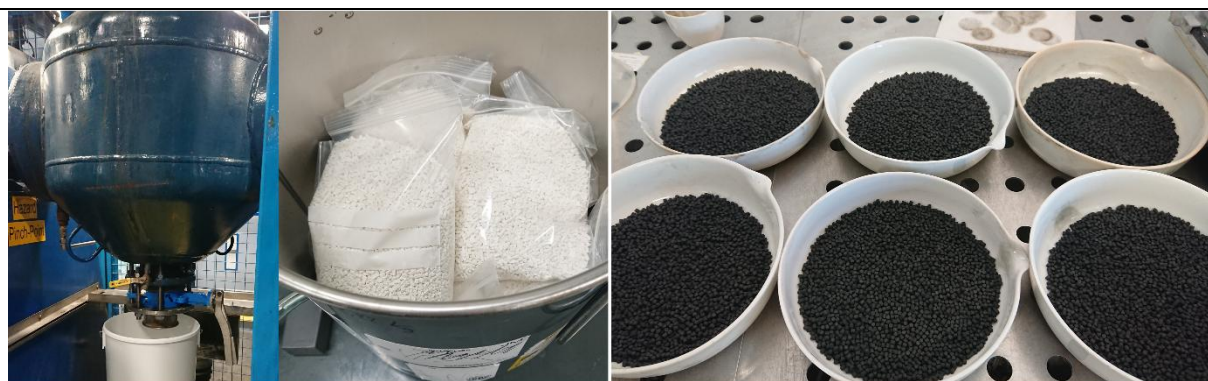
Scale up of the \text{MgCl}_2 sorbent: discharge of the final product and packaging under inert atmosphere
